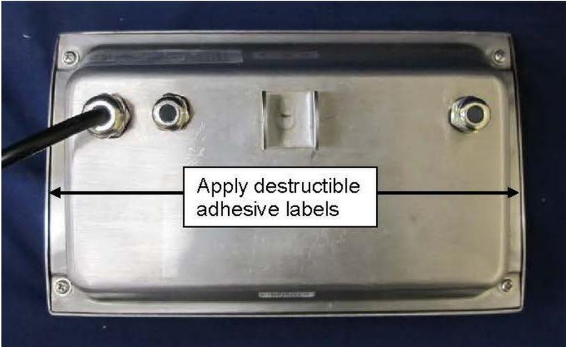
(b) Typical Sealing of PT Model PT253 Digital Indicator (variant 1)
