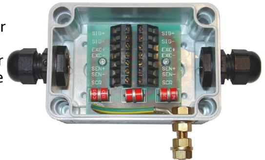
As stated above the earthing or grounding point is important to effective surge protection. The earth lug needs to be effectively bonded to the scale frame ground for load cell protection or indicator electrical ground for indicator protection.
